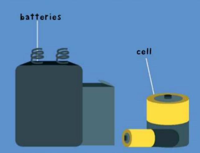
A cell is often shaped like a cylinder. sometimes the word "battery is used to refer to cells too. In this book, the word battery has to do with a box in which cells are joined together.
